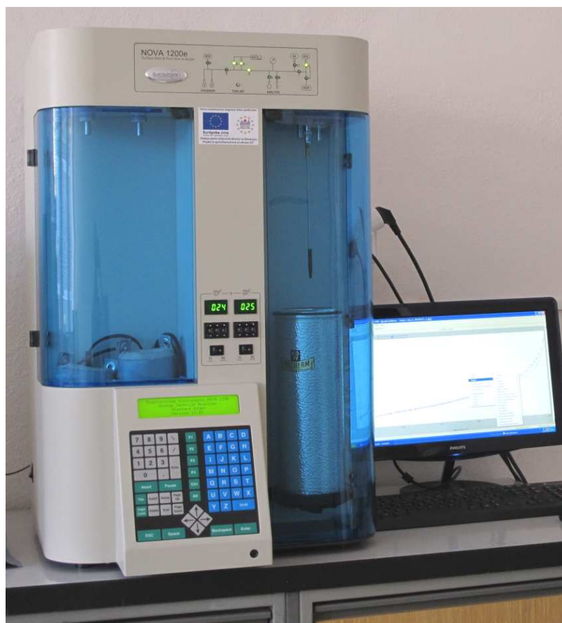
Surface area and pore size Analyzer Quantachrome NOVA 1200e (Quantachrome Instruments, USA)
