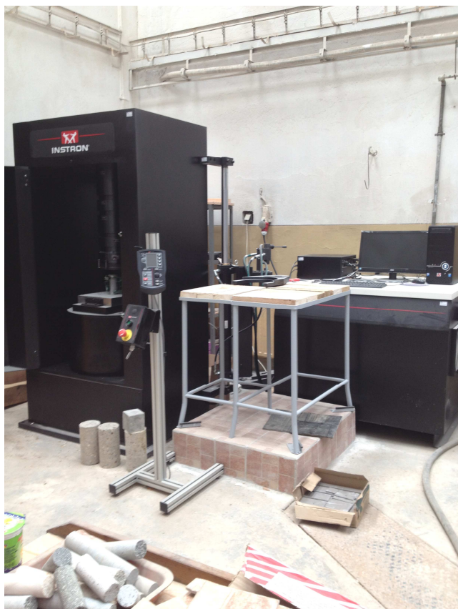
Hydraulic Press INSTRON 1000 RD, L 7072 up to 4,500 kN
