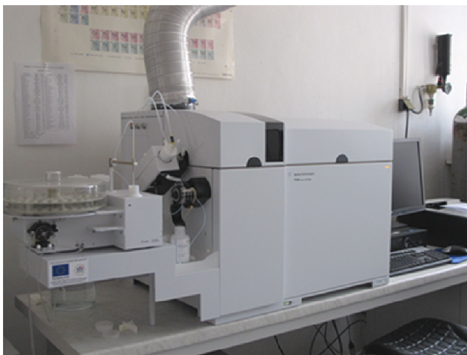
ICP-MS spectrometer Agilent 7700 for element detection in the range of 2–260 amu, a possibility ultratrace analysis with sensibility of ppt units
