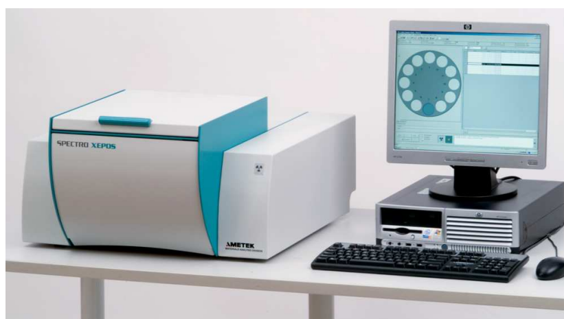
Spectro Xepos X-ray fluorescence spectrometer model XEPO3 (Spectro Analytical Instruments, Germany) with a range of _{11}\text{Na} – _{92}\text{U}
