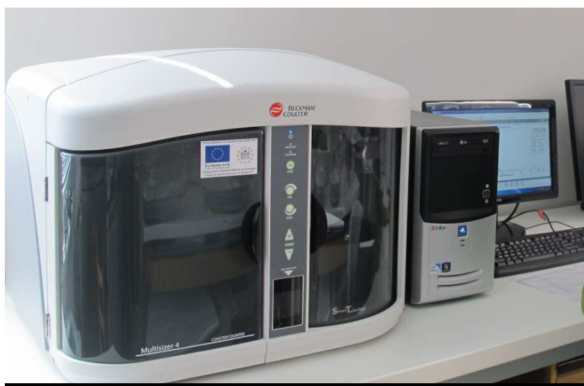
Particle size, volume and number distribution analyzer Beckman Coulter® Multisizer IV (Beckman Coulter, USA)
