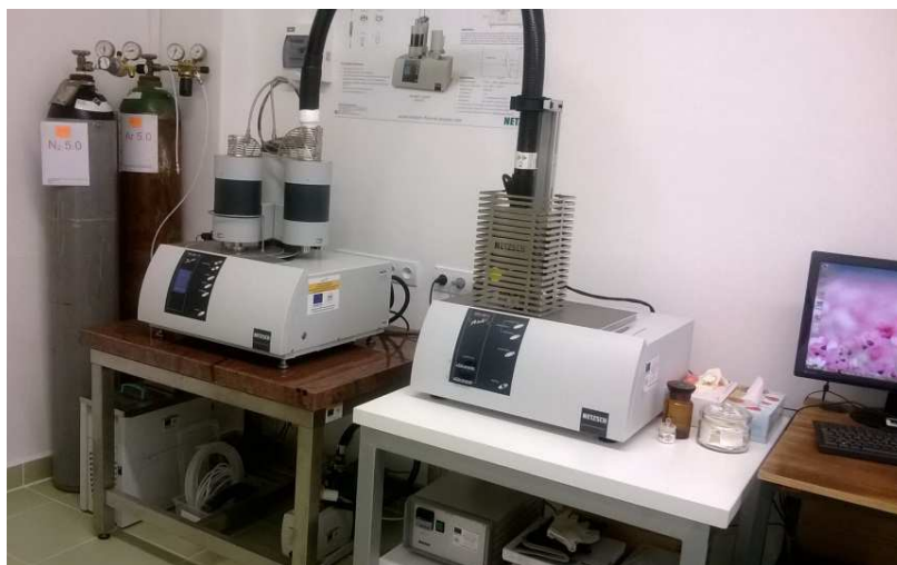
Thermal analyzer STA 449 F3 Jupiter (DTA/TG-DTG-DSC analyses) and mass spectrometer QMS 403 C Aëolos (Netzsch, Germany) for analysis of thermal decomposition products
